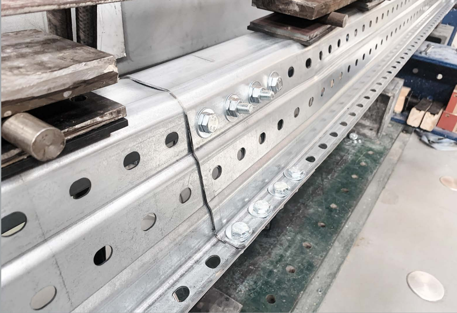
Layout 4 m Omegatek® 170x2,0 Simple amendment Deformation
